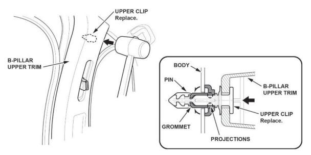
8. Pull back the top of the B-pillar upper trim to remove the upper clip from the body, then remove the trim.
