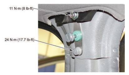
9.8. Remove the clip, and confirm the bracket hole is aligned with the original hole.
