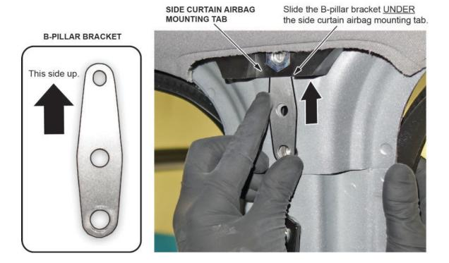
9.4. Install the new side curtain airbag mounting bolt, finger tight.
