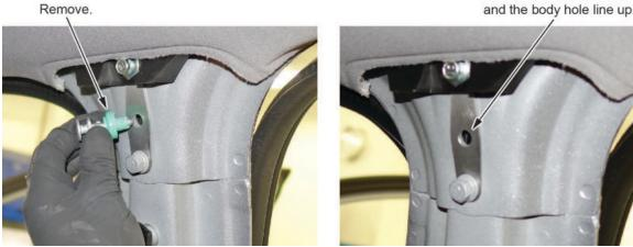
Be sure the bracket hole and the body hole line up.
