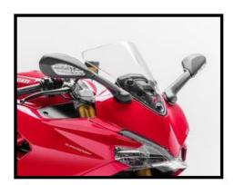
Ducati has elected to change both rear-view mirrors installed to the motorcycles affected by this Campaign. The new rear-view mirrors have been redesigned so as to improve visibility in the above conditions.
