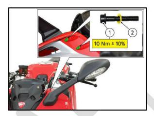
Please be reminded that the rear-view mirror opening/closing operation must be performed by applying a force perpendicular to the rotation axis of the mirror on its support. It is therefore important to pay special attention while rotating the mirror on its axis not to apply a longitudinal or transversal force.
