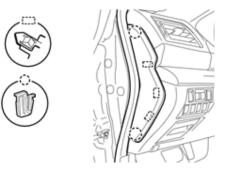
**Step 5:** Remove the philipps screw and release the 1 clip on the end portion of the trim shown in the photo. Then, **CAREFULLY** release and lower the lower IP trim panel by pulling it straight back toward you. **DO NOT** try to "peel" it up from the bottom. Leave all switches and the aspirator tube connected. Support the lower IP trim so there is no tension on the switch connections or harnesses.
