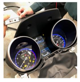
While the update is happening, the Yellow LED will blink on and off. When the update is complete, both the Green and Yellow LEDs will both come on solid. At this point, should the Red LED come on, repeat this (Step 10) again from the beginning. After successful completion, unplug the tool harness from the combination meter and the power supply from the wall outlet. This "resets" the tool.
