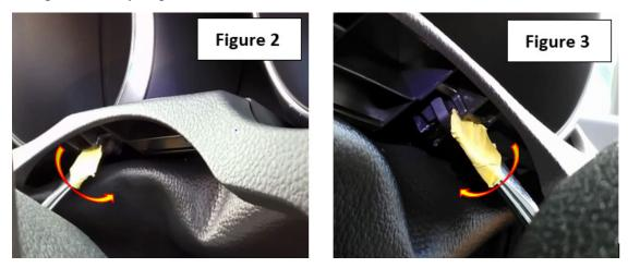
Once the bezel is loose, disconnect the trip reset button harness connector and put the piece aside. On Push Start models, LEAVE THE START SWITCH CONNECTED and just flip the bezel over toward the radio. Cover the bezel with a clean shop cloth to make sure does not scratch the audio unit face or any surrounding trim.
