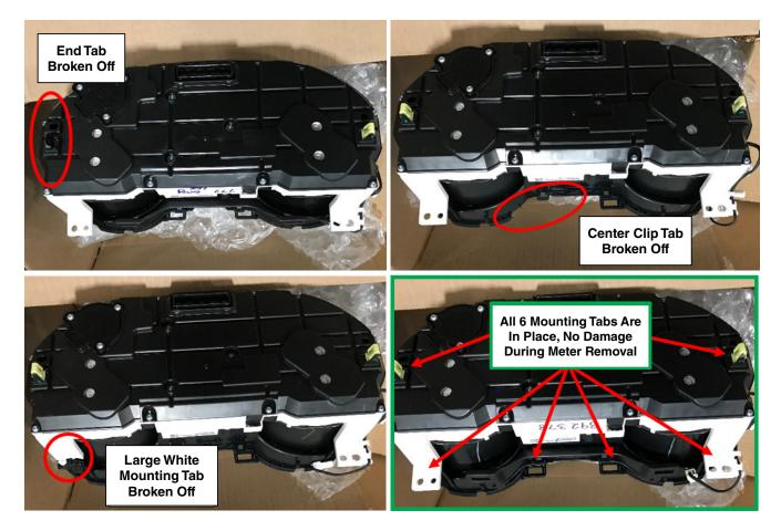
**Step 6: NOTE:** Previously, the removal procedure showed releasing the top claws on each end then grasping the bezel with the thumb and forefinger and pulling straight back to release the 2 center retaining clips.
