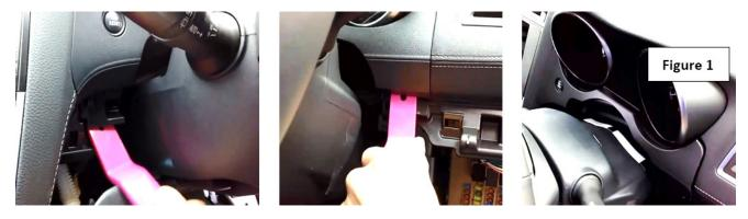
Use a flat-blade screwdriver with protective tape added shown in **Figure 2** and **3** below works well. A **CAREFUL** twist of the tool will release the clips. **NOTE:** These 2 center clips will likely require more effort to release the first time than in the future if necessary.
