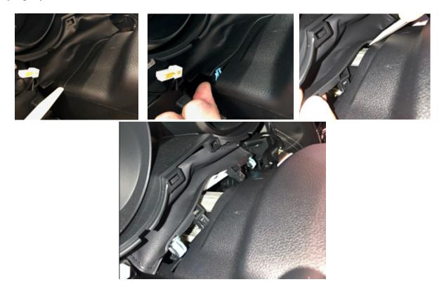
**Step 8:** Remove the 2- 10mm bolts from the underside of the visor and the 2 philipps screws on the bottom corners of the combination meter. **TIP:** Use a finger under the head of the screw to keep from dropping it inside the IP.
