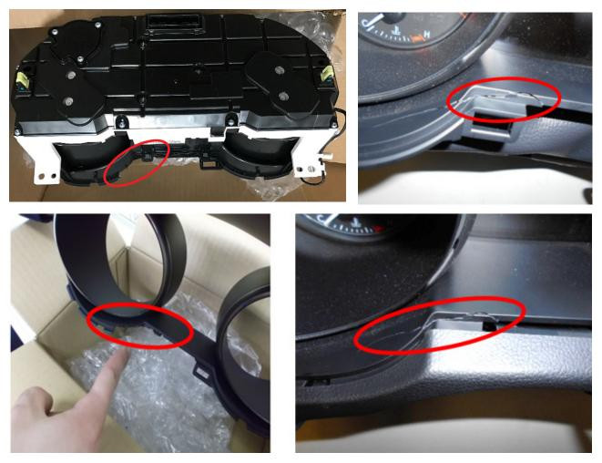
Use the photos below for reference when **CAREFULLY** removing the combination meter lower trim bezel.
