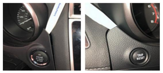
Release the lower claws on both ends of the bezel using a trim clip removal tool as shown.
