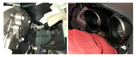
**Step 10:** Plug the AC adapter of the reprogramming tool into 120v AC "house current" and the combination meter harness connector into the meter. The meter will power up and illuminate completely. The tool's Yellow LED will illuminate. Press the black button to start the update. It takes about 70 seconds to complete.
