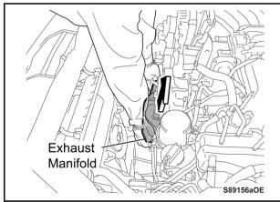
e) The worker in charge of engine lifting: Raise the exhaust manifold by hand and insert the 2 stud bolts on the engine to the holes in the exhaust manifold.
