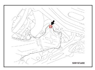
f) The other worker: Temporarily install a *NEW* nut to the exhaust manifold from underneath the vehicle.
