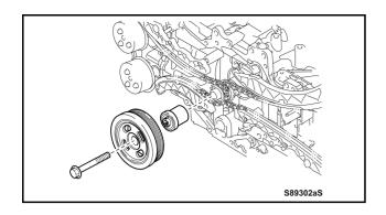
c) Remove the bolt, the crankshaft pulley and the spacer.
