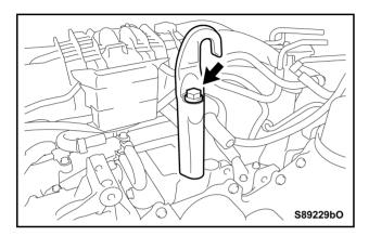
8. REMOVE ENGINE SLING DEVICE AND ENGINE HANGER
