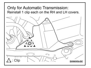
d) Reinstall 1 clip each on the left and right engine under covers.
