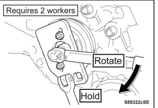
f) While another worker holds the crankshaft pulley in place using SST, install the bolt.
