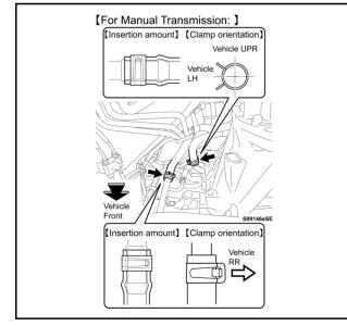
7. RECONNECT HEATER WATER HOSES (for Manual Transmission)
