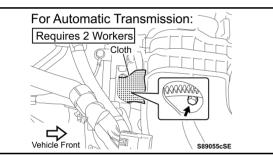
1. REMOVE TORQUE CONVERTER STOPPER (for Automatic Transmission)
