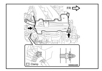
**19. REINSTALL V-RIBBED BELT TENSIONER** ASSEMBLY
