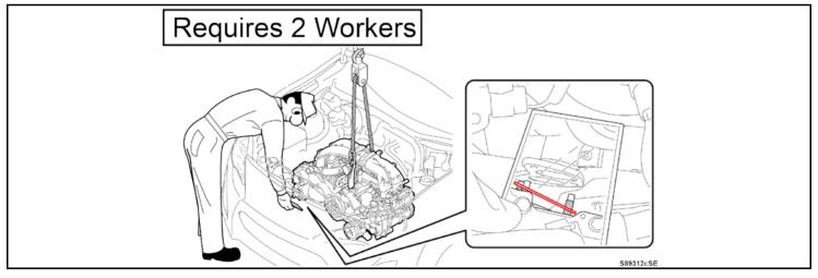
d) The other worker: Align the left side stud bolt on the engine block with the exhaust manifold hole, from the vehicle underside.
