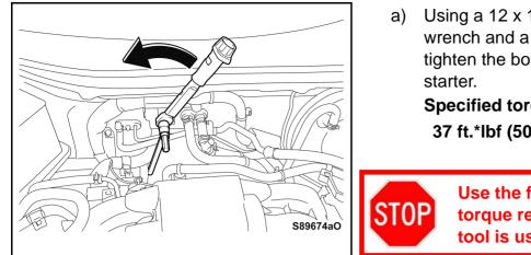
a) Using a 12 x 14 mm (0.47 x 0.55 in.) offset wrench and a 12 mm (0.47 in.) hexagon socket, tighten the bolt on the upper portion of the
