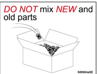
f) Remove the valve spring, mark and then store it in a separate container so as not to reinstall it in error.
