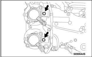
d) Reinstall the 2 wire harness brackets with the 2 bolts.
