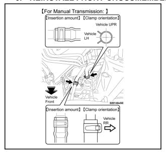
7. RECONNECT HEATER WATER HOSES (for Manual Transmission)
