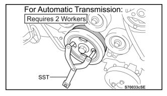
3. REINSTALL DRIVE PLATE AND TORQUE CONVERTER SETTING BOLTS (for Automatic Transmission) (Requires 2 Workers)
