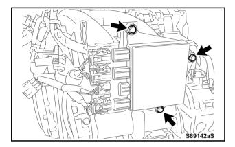
b) Reinstall the injector driver with the 3 bolts. **Specified torque:**
