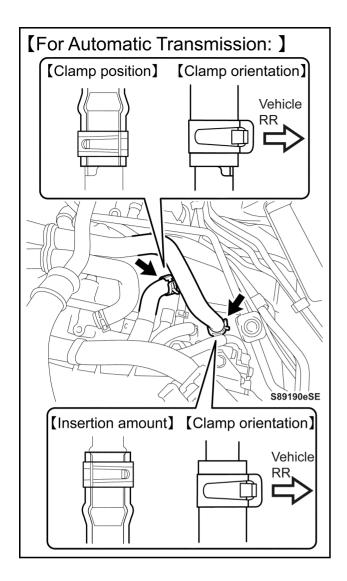
10. RECONNECT TRANSMISSION OIL COOLER HOSE NO. 3 AND HEATER WATER HOSE OUTLET B (for Automatic Transmission)
