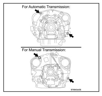
b) Reinstall the 2 transmission coupling bolts.
