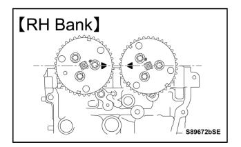
c) Align the alignment marks to set both camshafts to no lift positions.
