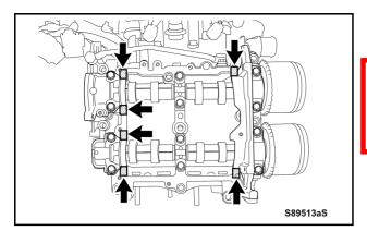
Completely remove any excess seal packing outside the camshaft caps.
