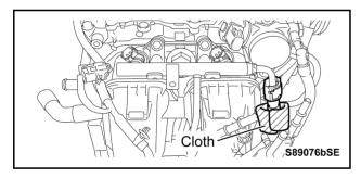
d) Wrap cloth under the area where the pipes are being disconnected to catch the fuel that will trickle out.
