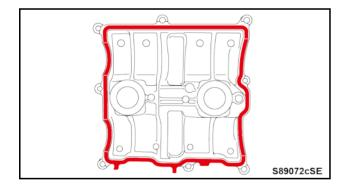
c) Install a **NEW** rubber gasket.
