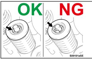
p) Visually confirm that the retainer locks are securely engaged with the valve.
