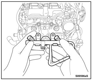
g) While holding the delivery pipes and the injector firmly in one, pull out the injector from the intake manifold.
