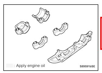
b) Apply thin coat of engine oil to 5 camshaft caps on the mating surfaces of the journals.
