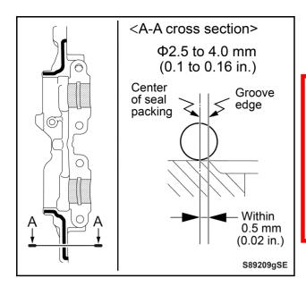
d) Using the sealer gun, apply seal packing to the front camshaft cap.
