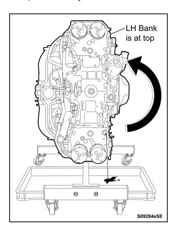
b) Rotate the engine stand until the LH Bank (No. 2 and No. 4 cylinders) is at top.
