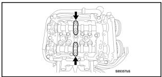
c) Remove the 2 center camshaft caps.
