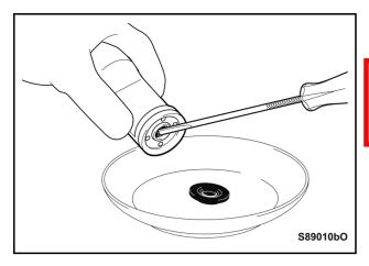
e) Detach and remove the retainer and the retainer locks from the magnets.
