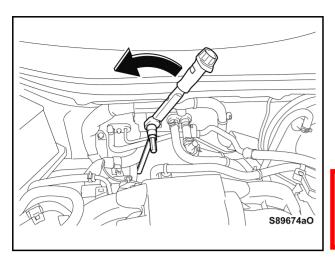
a) Using a 12 x 14 mm (0.47 x 0.55 in.) offset wrench and a 12 mm (0.47 in.) hexagon socket, tighten the bolt on the upper portion of the starter.
