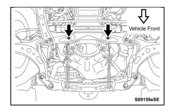
g) Slowly lower the engine and lead the engine mounting stud bolts through the cross member holes.
