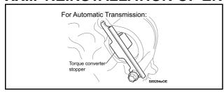
1. REMOVE TORQUE CONVERTER STOPPER (for Automatic Transmission)
