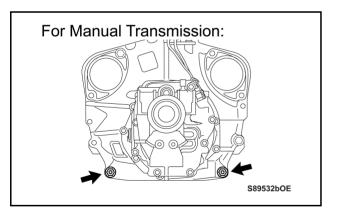
b) Reinstall the 2 nuts.Specified torque:37 ft.\*lbf (50 N\*m, 510 kgf\*cm)
