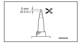
c) Cut off approximately 5 mm (0.2 in.) from the tip of a sealer gun nozzle.
