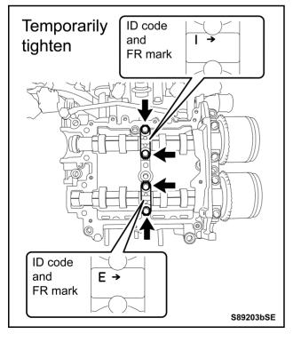
g) Check the identification code and front mark on each center camshaft cap, set the 2 caps, and temporarily reinstall them with the 4 bolts.
