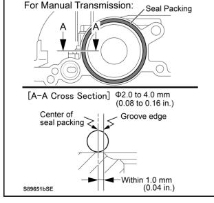
Each component must be attached within 5 minutes of seal packing application, and all bolts must be tightened to the specified torque within 15 minutes of the application.
