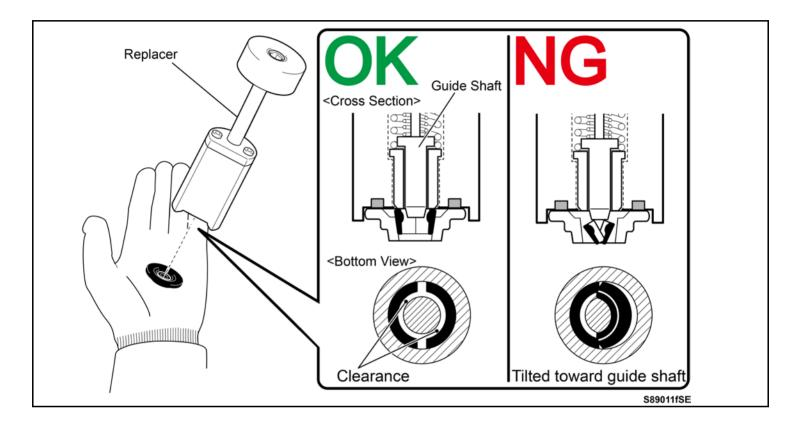
n) While covering the replacer by hand, set the replacer on the valve. If the replacer is not covered by hand, a retainer or retainer lock attracted to the magnets may accidentally fall into the engine.
