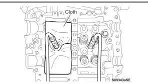
c) Remove the cloth from cylinder No. 1, and then place it to cover cylinder No. 3 as shown.
