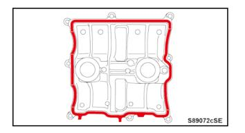
c) Install a **NEW** rubber gasket.
