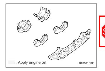
Apply thin coat of engine oil to 5 camshaft caps b) on the mating surfaces of the journals.
