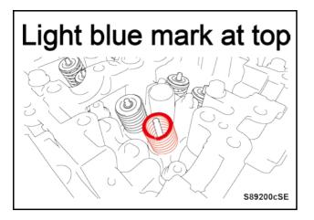
h) Set a *NEW* valve spring on the cylinder head with its light blue mark side facing upward.
