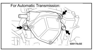
g) Reinstall the vacuum pump with the 3 bolts.
