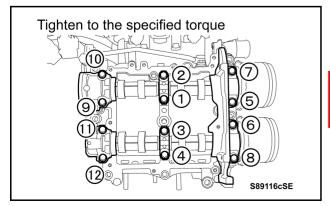
j) Set the 2 rear camshaft caps and then temporarily tighten the 4 bolts.
