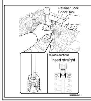
a) Insert the retainer lock check tool to the valve stem tip, and then lightly tap it to properly seat the retainer locks.
