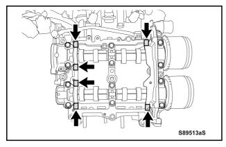
I) Completely remove any excess seal packing outside the camshaft caps.
