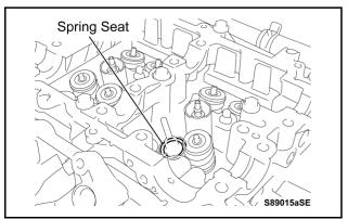
g) Check that the spring seat (can be installed facing either direction) is set on the engine.
