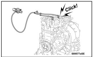
c) Connect the air hose to the 2 air adaptors.
