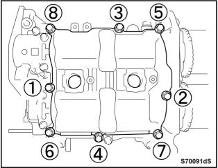
f) Set the cylinder head cover RH, and install it by uniformly and gradually tightening the 8 bolts in the specified order in several passes.
