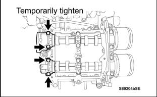
j) Set the 2 rear camshaft caps and then temporarily tighten the 4 bolts.
