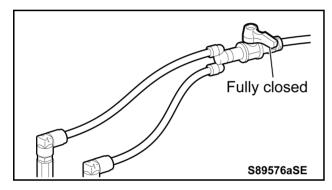
b) Confirm that the valve is fully closed.
