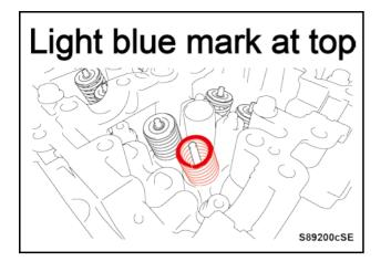
Set a NEW valve spring on the cylinder head with its light blue mark side facing upward.
