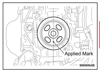
c) Confirm that the mark applied on the crankshaft pulley is not in any position other than as shown in the illustration.
