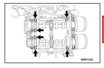
Completely remove any excess seal packing outside the camshaft caps.
