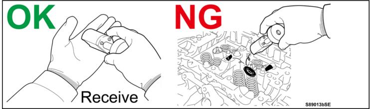
o) Set the replacer guide shaft end on the valve stem end as shown, and push the replacer straight downward until the spring is compressed by approximately 12 mm (0.47 in.), to install the retainer and the retainer locks. Be careful when removing the tool, as the retainer locks may not be installed properly.
