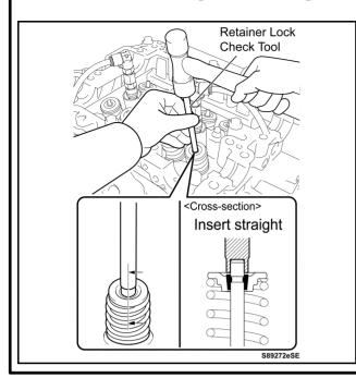
a) Insert the retainer lock check tool to the valve stem tip, and then lightly tap it to properly seat the retainer locks.
