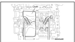
Remove the cloth from cylinder No. 1, and then place it to cover cylinder No. 3 as shown.
