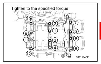
k) Uniformly and gradually tighten the 12 bolts in the specified order in several passes.
