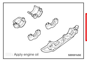
Apply thin coat of engine oil to 5 camshaft caps on the mating surfaces of the journals.
