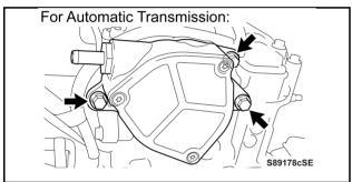
g) Reinstall the vacuum pump with the 3 bolts.Specified torque:12 ft.\*lbf (16 N\*m, 163 kgf\*cm)
