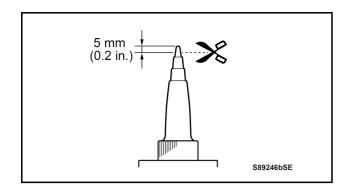
c) Cut off approximately 5 mm (0.2 in.) from the tip of a sealer gun nozzle.
