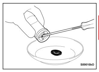
e) Detach and remove the retainer and the retainer locks from the magnets.
