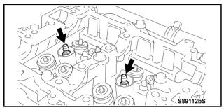
a) Attach the 2 air adapters by hand.
