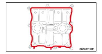
c) Install a **NEW** rubber gasket.
