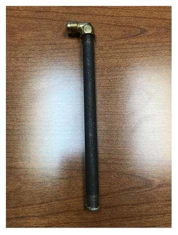
The image to the left is the supplied piece which will replace the flared coupler and create a rigid pipe section throughout the entire burner box of the 2 burner cooktop. The 90 degree elbow will be oriented outside of the cooktop burner box.
