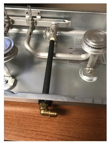
Note: in order to install the new pipe section, the 90 degree elbow can be fed through the grommet at the back of the burner box, or for easier installation, the entire 2 burner cooktop can be removed from the pullout tray by removing the screws from the side flange. (Cooktop removed in this image for visual clarification.)
