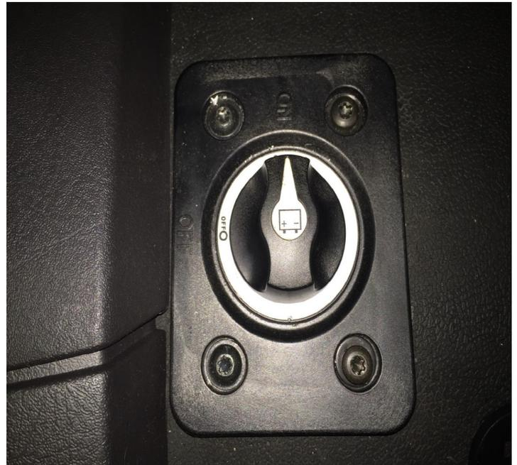
3.) While holding the bottom right button down, turn the master power switch to the ON position as shown in figure 3. Once the screen displays “booting” release the button. A series of arrows will appear on the righthand side of the screen. Push the button next to the bottom arrow pointing to the right and the arrow will turn green. Push the same button a second time and the program will update. The display screen will go blank and say “booting”.
