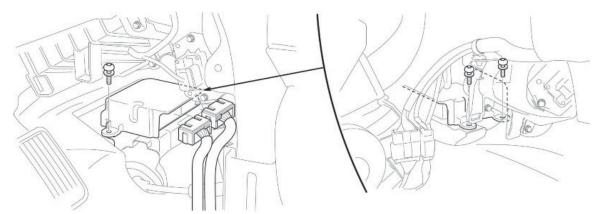
7. Mark and remove the old SRS unit and install the new unit.
