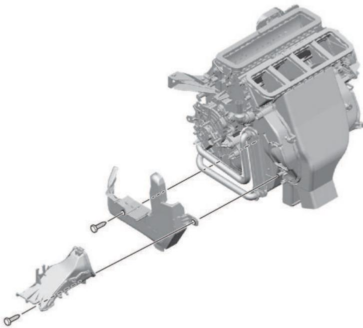
8. Remove the air duct.
