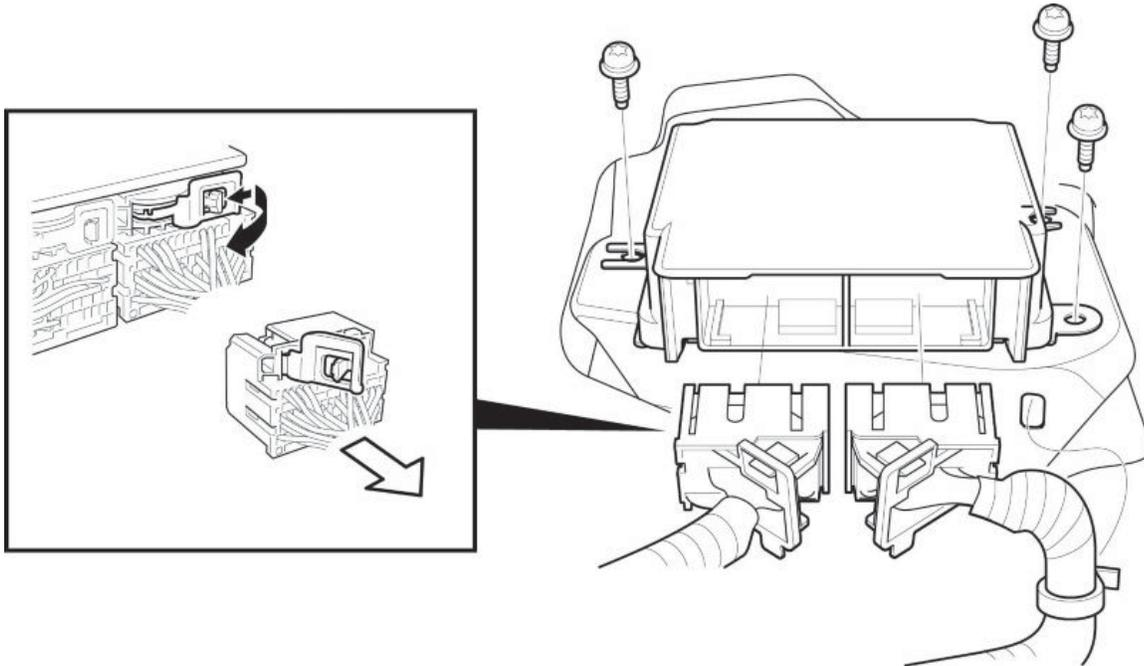
10. Install the new SRS unit, tighten the new bolts to the specified torque 11 Nm (8 lb-ft) in the numbered sequence shown.
