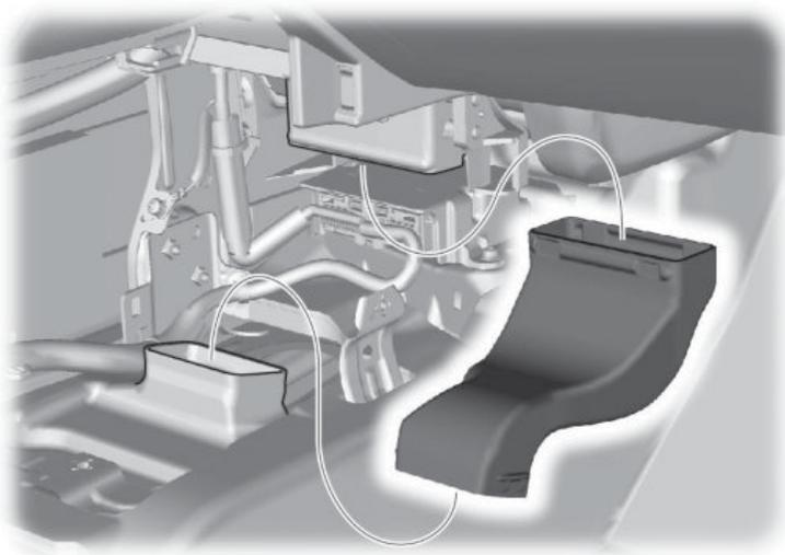
9. Disconnect the SRS unit connectors, remove and discard the three T30 TORX bolts securing the SRS unit.
