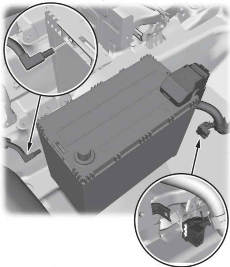
5. Disconnect the 12-volt battery positive terminal.
