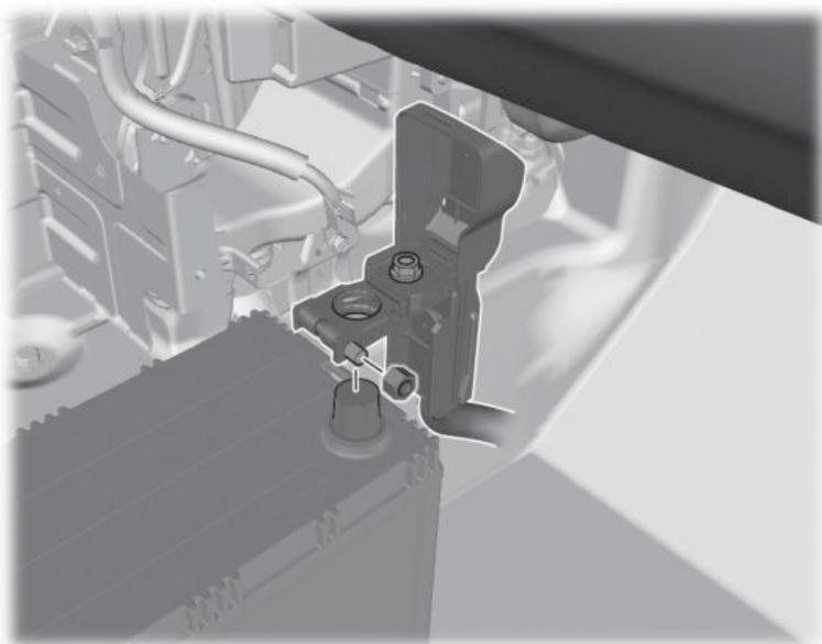
6. Remove battery set plate and drain tube.
