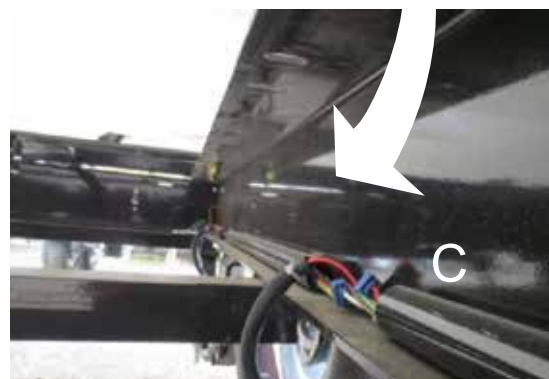
Figure 17. Wire Harness Connections
