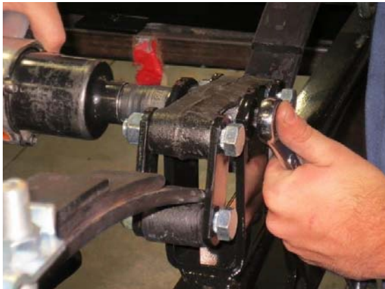
Figure 6. Loosening Axle Hex Nuts
