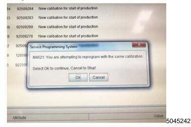
Note: If the Same Calibration/Software Warning is noted on the SPS controller screen, select "OK" and continue programming.
