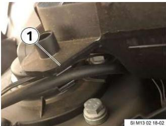
Unlock the washer hose clip and remove the washer hose from the lower cowl cover (1).
