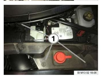
Remove screws for the upper bulkhead cover and the cover for the B+ terminal (1).
