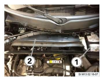
Remove the B+ cover (1) and then remove the upper bulkhead cover (2).
