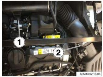
Remove screw (1) and intake hose clamp (2) from the intake air pipe.
