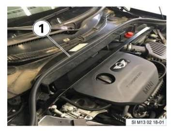
Remove the rear engine to hood seal
