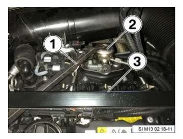
• Using an appropriate length pry bar (1), apply pressure to the top of the high pressure pump (2) using the strut brace (3) as a fulcrum.
