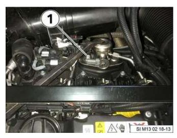
• Remove the right side screw for the high pressure pump (1).
