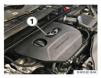
Remove the engine acoustic cover (1)
