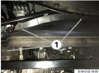
Remove screws (1) for the upper bulkhead cover.
