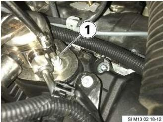
Remove the left side screw for the high pressure pump (1).
