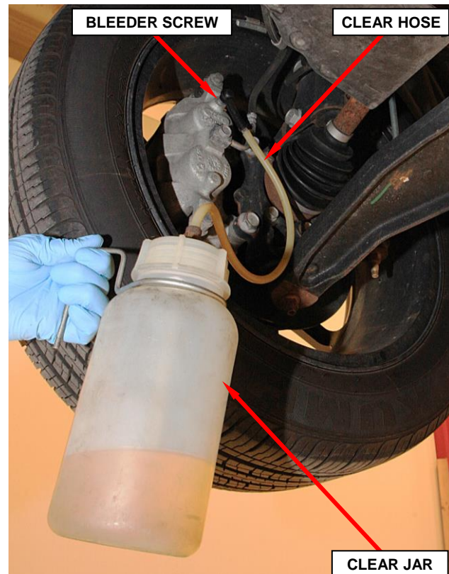
Figure 2 – Brake Bleeding Equipment
