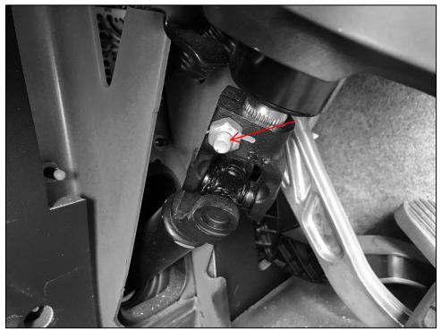
Figure 1, Steering Pinch Bolt
