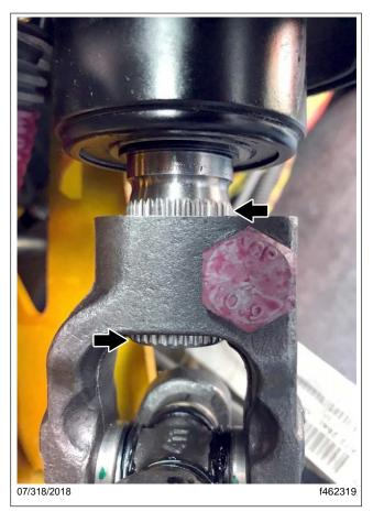
Fig. 2, Steering Shaft Splines
