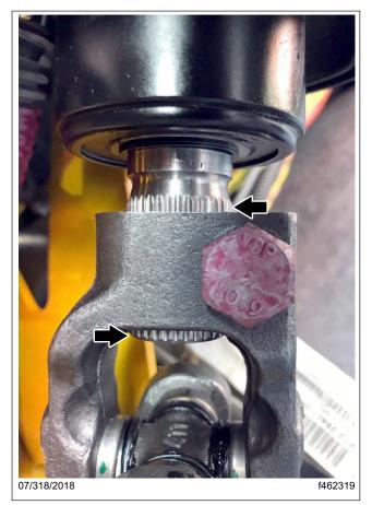
Fig. 1, Steering Shaft Splines
