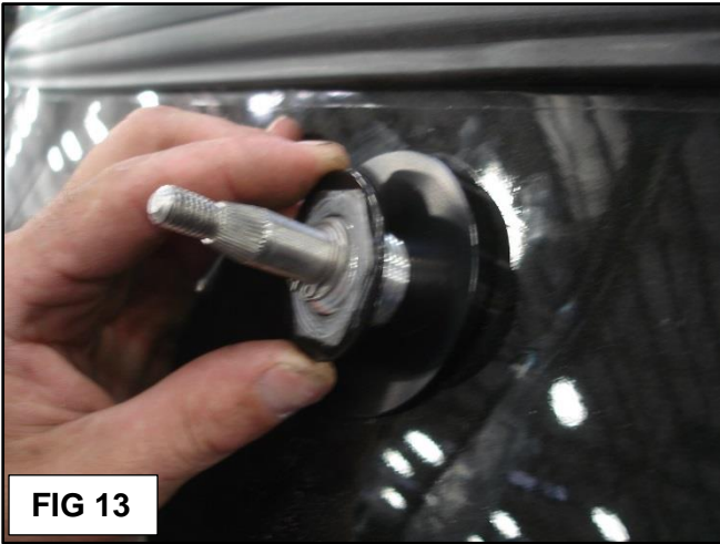
FIG 13: Install the flat washer on each wiper stud.
