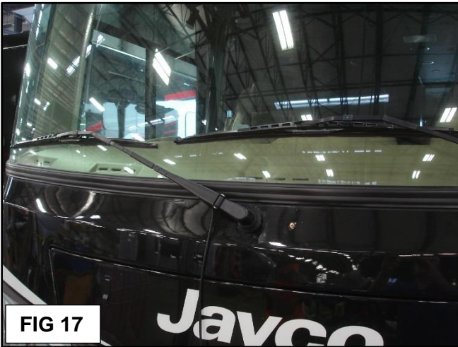
FIG 17: Install the old wiper blade assemblies on to the new arms from the kit. Install the completely assembled arms and blades on to the wiper studs. Make sure the wiper blades click on to the wiper arms. Make sure the blades match the parked position taped off in Step 2.
