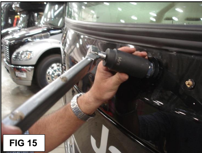
FIG 15: Torque the 33mm nut to 15 ft/lbs with the torque wrench using the 1-5/16" socket.
