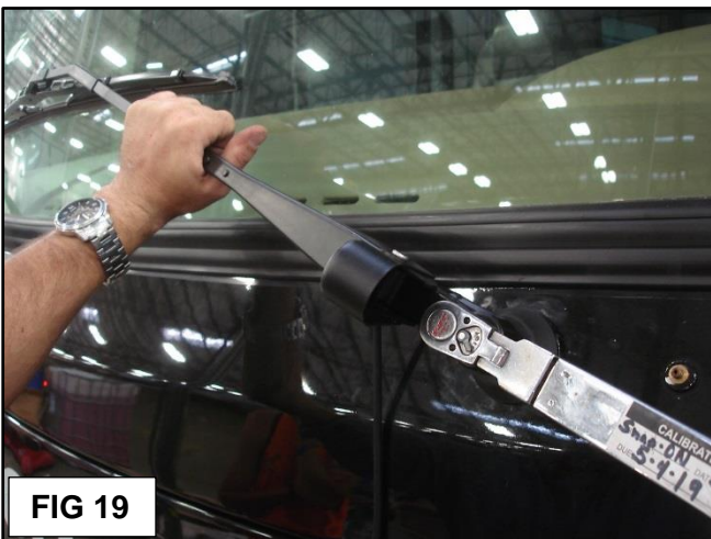
FIG 19: Torque the 13mm flanged nuts on the wiper arms to 15 ft/lbs each. Wait 30 minutes and re-torque the nuts again to 15 ft/lbs each. Wiper system should NOT be powered on until this step has been completed.
