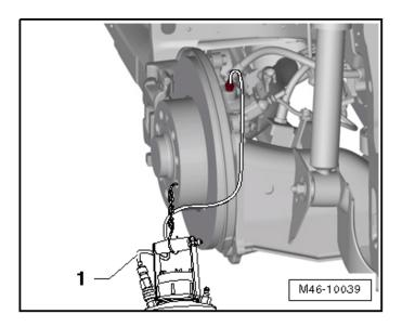
Connect the bleed hose <1> from the bleeder bottle to one of the calipers being replaced and open the bleed valve.
