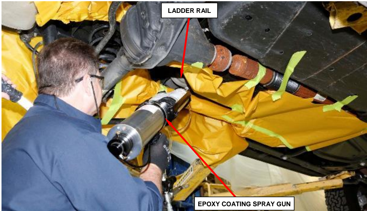
Figure 9 – Apply Epoxy Coating to Ladder Rail from Underside of Vehicle
