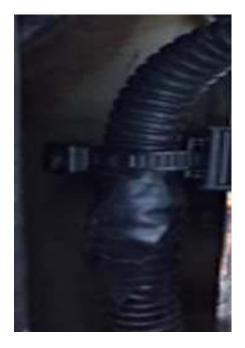
Install end clip wire tie (PN 19-11-3473) on the harness and secure to the edge of the coolant surge tank as shown below. Trim off wire tie end after securing around the harness.
