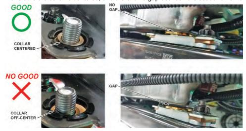
17. Install and hand tighten the nuts, then torque them to 52 N·m (38 lb-ft) in the sequence shown.
