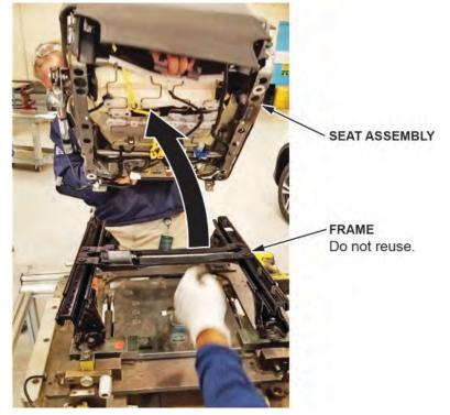
12. Make sure the new frame is for the driver's side, and replace the original driver's seat frame.
