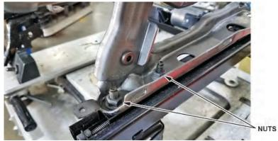
11. Make sure nothing is connected to the frame, then slowly lift the seat and set it aside.
