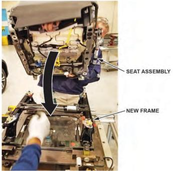
16. Make sure the collar is centered, and there is no gap between the seat and frame.
