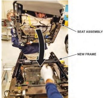
14. Install and hand tighten the 2 torx bolts into the rear-right corner, then the 2 nuts in the remaining 3 corners.
