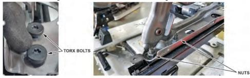
15. Torque the torx bolts and nuts to **30 N·m (22 lb-ft)** in the sequence shown.
