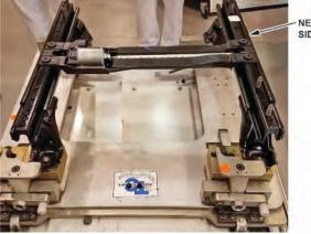
NEW DRIVER'S SIDE FRAME 13. Slowly place the driver's seat onto the new frame.
