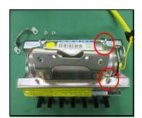
5. Loosen, but do not remove, the circled nuts.
