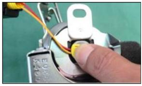
20. Press the wiring harness connector firmly into the electrical connector socket.
