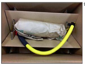
Package the old inflator, with its wiring harness still attached, into the box that previously contained the new inflator. Ensure the old inflator is correctly wrapped, using the wrapping that came with the new inflator, to protect the old inflator from damage during shipping.
