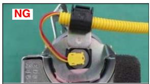
**CAUTION:** Do not connect the wiring harness in the incorrect direction.
