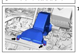
7. INSTALL AIR CLEANER INLET (Highlander Only) a. Install the air cleaner inlet with the 2 bolts.
