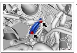
1. INSTALL No. 2 SURGE TANK STAY a. Install the side stay with the 2 bolts.
