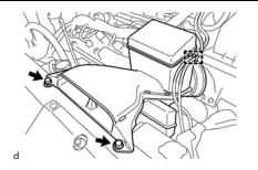
8. INSTALL THE AIR CLEANER INLET (Sienna Only) a. Install the air cleaner inlet with the 2 bolts.
