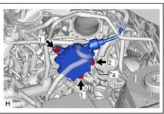
d. Install the 3 **NEW** bolts with adhesive applied. Torque: 15 lbf.ft {21 N·m, 214 kgf·cm}
