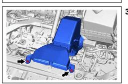
3. **REMOVE THE AIR CLEANER INLET (Highlander Only)** a. Remove the 2 bolts and the air cleaner inlet.
