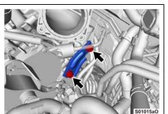
3. REMOVE No. 2 SURGE TANK STAY a. Remove the 2 bolts.
