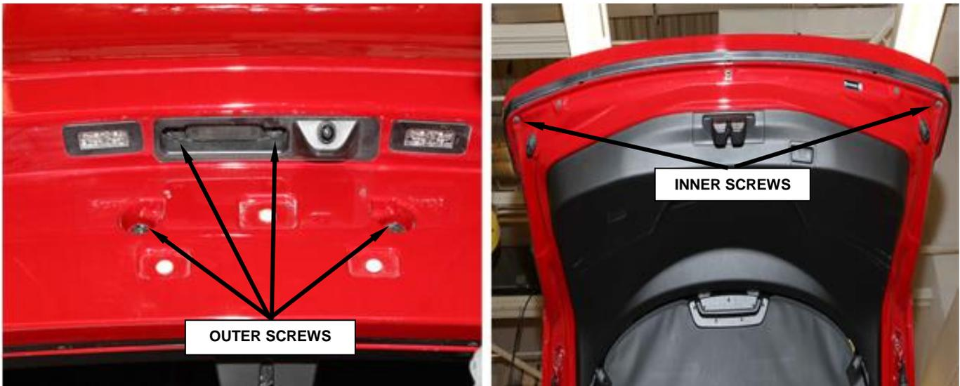
Figure 26 – Fastening Screws
