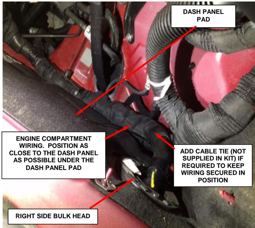
**Figure 14 – Engine Wiring Routing**
