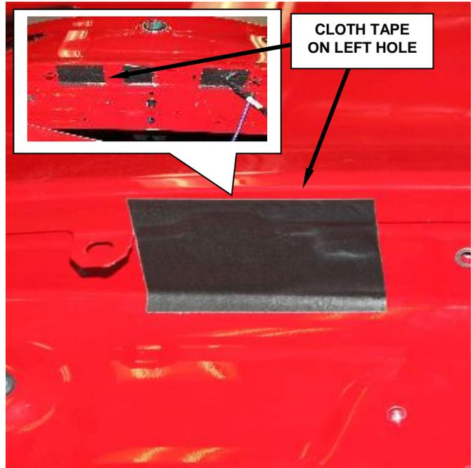
**Figure 27 - Cloth Tape to Left Side of Liftgate**
