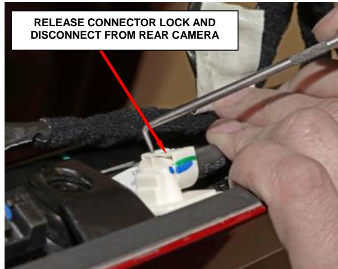
**Figure 35 – Rear Camera Connection**
