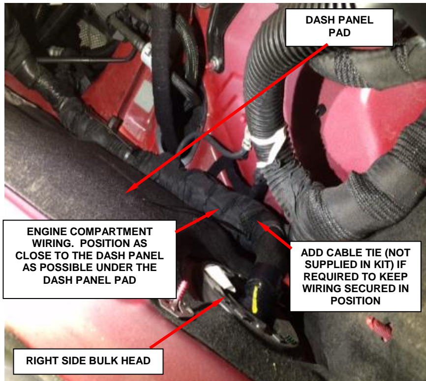
Figure 14 – Engine Wiring Routing
