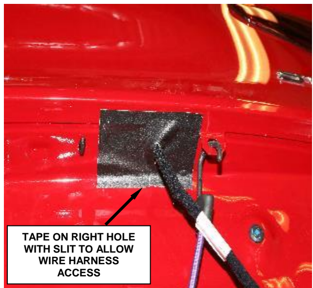
Figure 29 - Cloth Tape to Right Side of Liftgate
