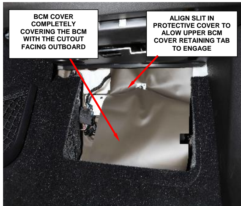
Figure 25 – Protective Cover Installed
