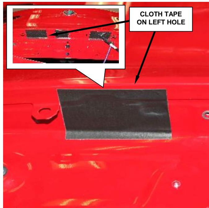
Figure 27 - Cloth Tape to Left Side of Liftgate
