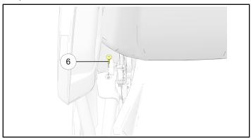
Deflect floor pan slightly upward to gain access to horizontal rear seat fastener ③.
