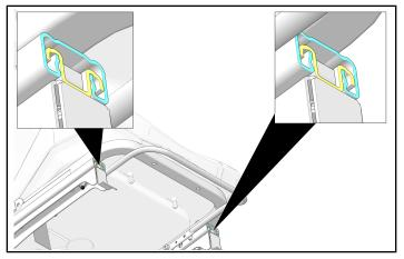
5. Carefully install seat assembly into vehicle.
