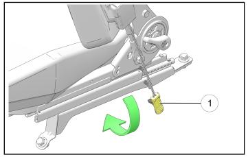
Connect the seatbelt switch electrical plug (connected to the harness) to the connector mounted to the seat frame. Gently pull on connector to ensure locking tab is engaged.
