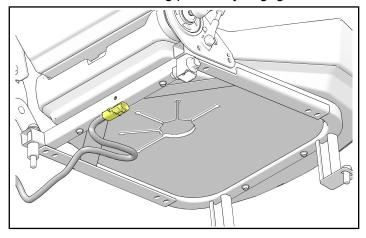
7. Using a 15 mm socket, loosely install vertical rear seat fastener ②.
