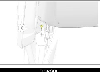
TORQUE Floor Pan Fastener: 65 in-Ibs (7 Nm)
