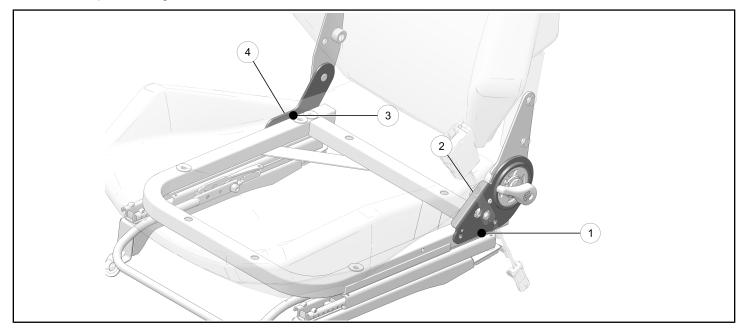
• If all welds are present on the driver-side seat base frame, perform the Seat Slider Test on page 11.
