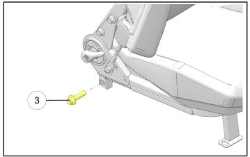
10. Align the front seatbase mounting holes with the vehicle and loosely install the two front seat fasteners ①. Leave fasteners loose to ease final assembly of the rear fasteners.
