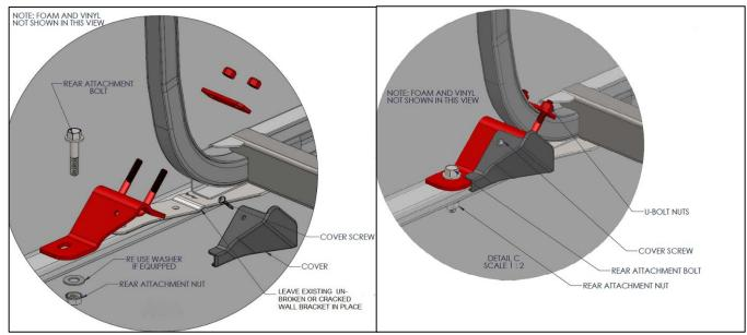
Figure 3: Bracket Installation (Driver's Side Shown) – 26 Inch, 36 Inch, and 39 Inch Seats
