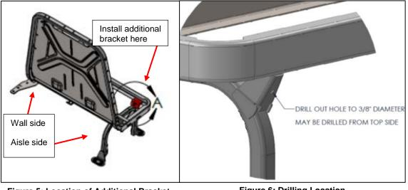
Figure 5: Location of Additional Bracket (Driver's Side Shown)
