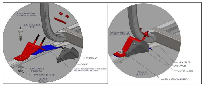
Figure 4: Installation with Safe Spacer (Driver's Side Shown) – 26 Inch, 36 Inch, and 39 Inch Seats
