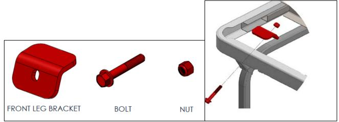
Figure 7: Additional Parts for 30 Inch and 32 Inch Seats
