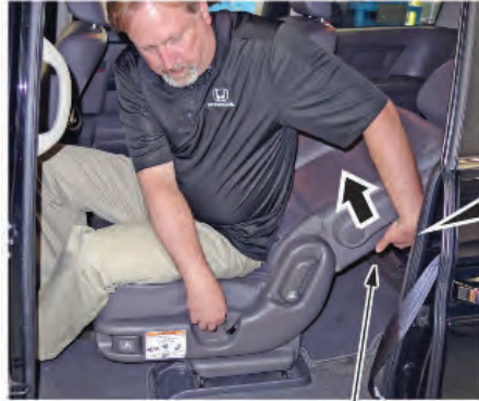
Lift the seat-back to free it from the trim panel if necessary.
