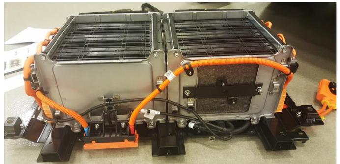
15. Reinstall the watertight cover to the Sub High Voltage Battery Pack.
