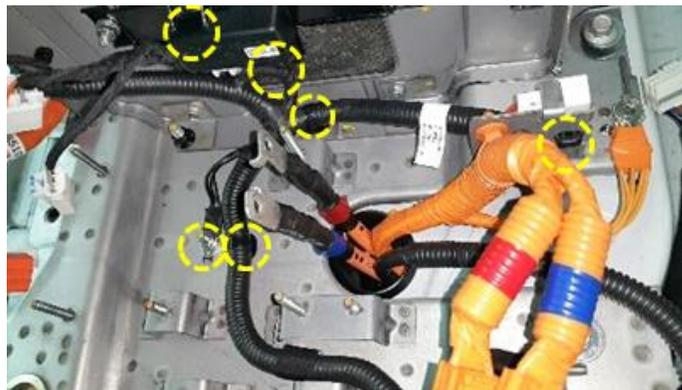
36. Install the new MAIN BMS WIRING 37517-E6520QQH.
