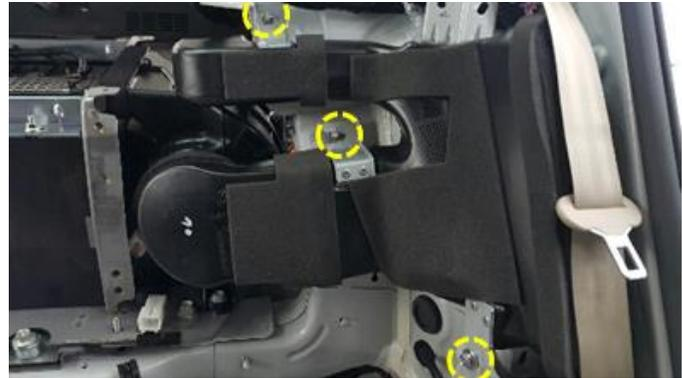
26. Remove the mounting screws and cooling duct (G).
