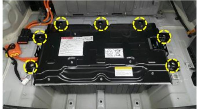
6. Remove the mounting bolts and cover from the Sub High Voltage Battery Pack.
