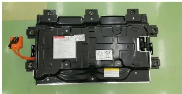
18. Loosen the mounting bolts and remove the front cover (D) of the Main High Voltage Battery Pack.
