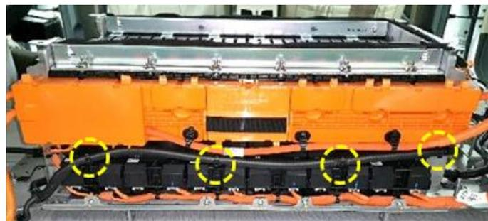
34. Remove the mounting clips, VPD nuts, and ground bolt.
