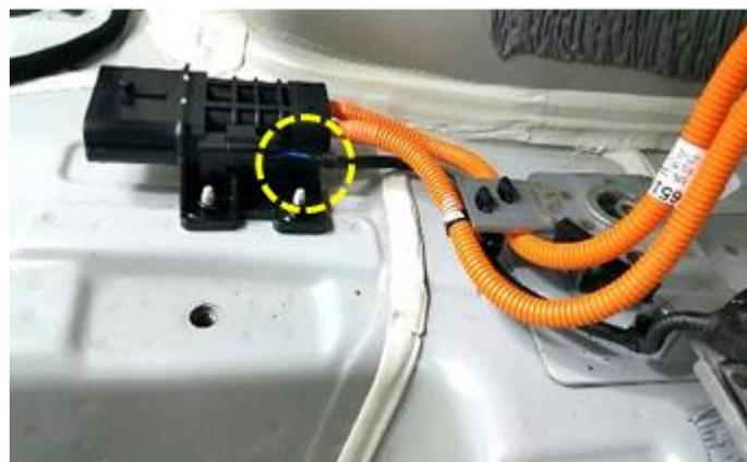
33. Remove the main wiring harness mounting clips.
