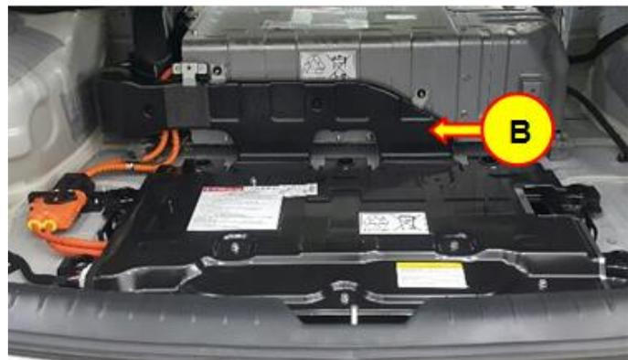
5. Remove the mounting bolts and Sub High Voltage Battery Pack from the vehicle.
