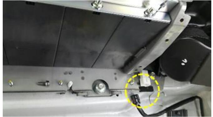
25. Remove the cooling duct mounting bolts and nuts.
