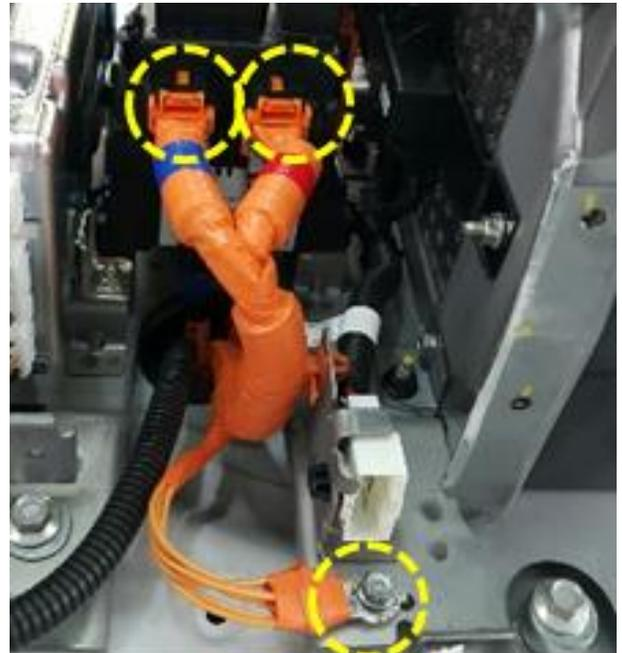
23. Remove the inverter power positive and negative cable terminals.
