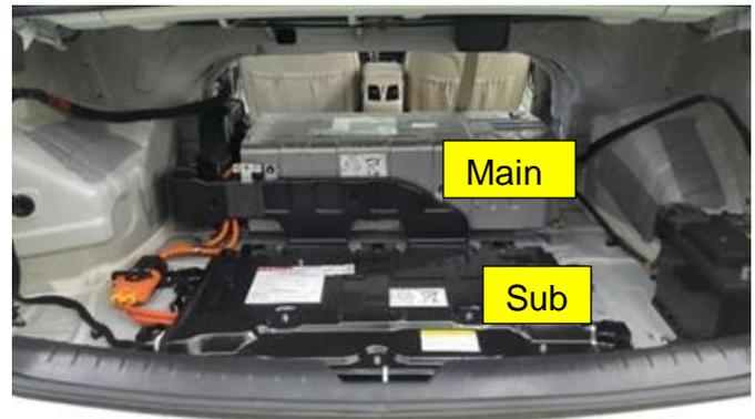
3. Disconnect the BMS and high voltage connectors (A) from the Sub High Voltage Battery.
