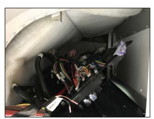
Figure 6: Back of PC Boards After Side Cushion is Removed
