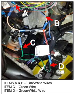
Figure 2: Current Harness Installation
