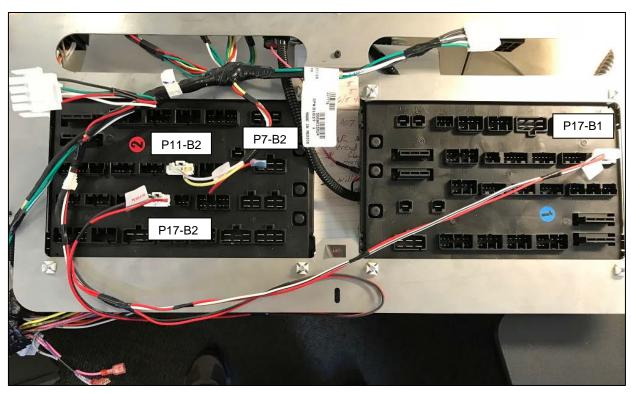
Figure 7: Rear of PC Boards Showing Connections, Only
