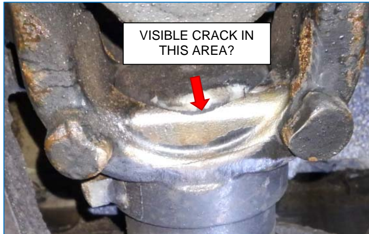
Figure 12: Potential Crack Area
