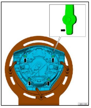
If a pin is damaged or has been lost, it can be replaced with a locking pin from the bag of spares included.
