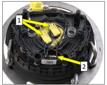
Subsection 4 – Renewing inflator, four spoke steering wheel, with vibration absorption
