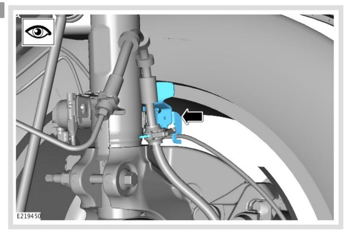
Locate the front left brake hose support bracket.
