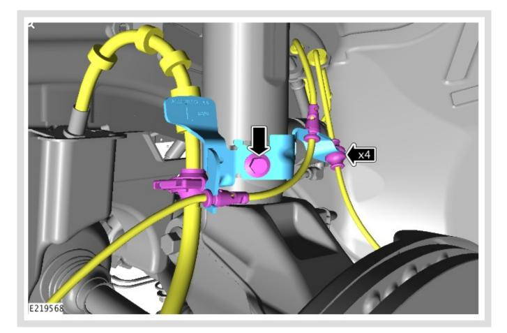
Replace the brake hose support bracket.
