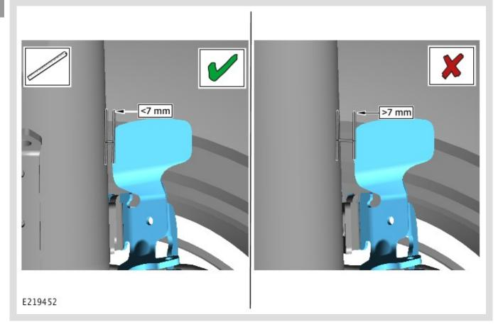
Measure and record the gap between the brake hose support bracket and the shock absorber.
