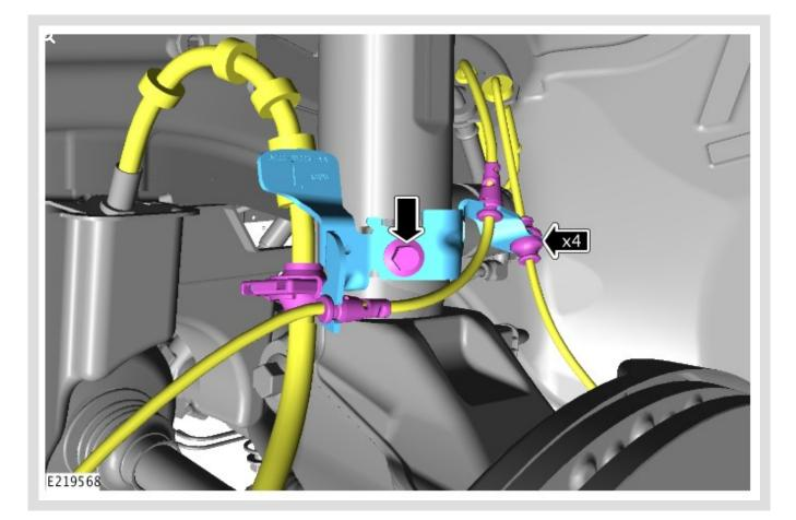
Replace the brake hose support bracket.
