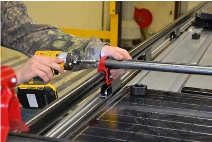
12. Put Loctite on T-bolts when reattaching the hand nuts on side rails. Protect and clean any excess Loctite from motorhome.
