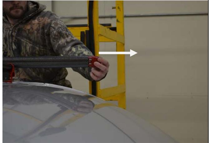
15. On the forward rail: Use a carriage bolt to reattach the red plastic saddles to the side roof rails. Slide the head of carriage bolt through the side roof rails. Tighten down with a washer and nylock nut.
