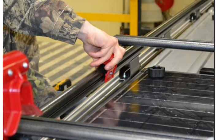
11. Reattach red plastic saddles to adjustable rails. Secure using the two screws from the supplied hardware kit.
