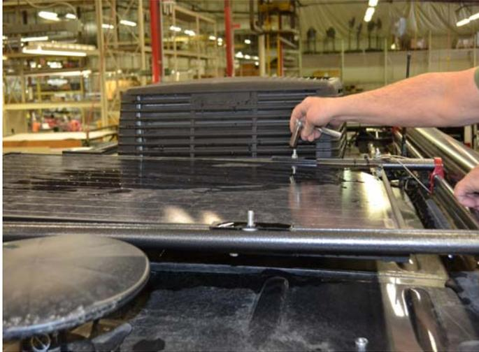
2. If your motorhome is equipped with security cables, remove cables and discard the cable and two attachment bolts.
