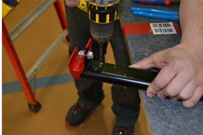
6. Attach the support bracket to the roof rail with two rivets.
