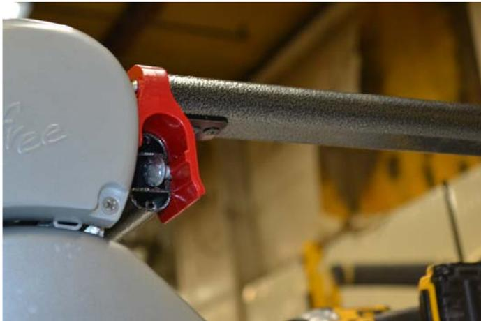
16. Reattach the red plastic bullet caps to the forward rails. Reinsert screws and tighten with a screw gun.
