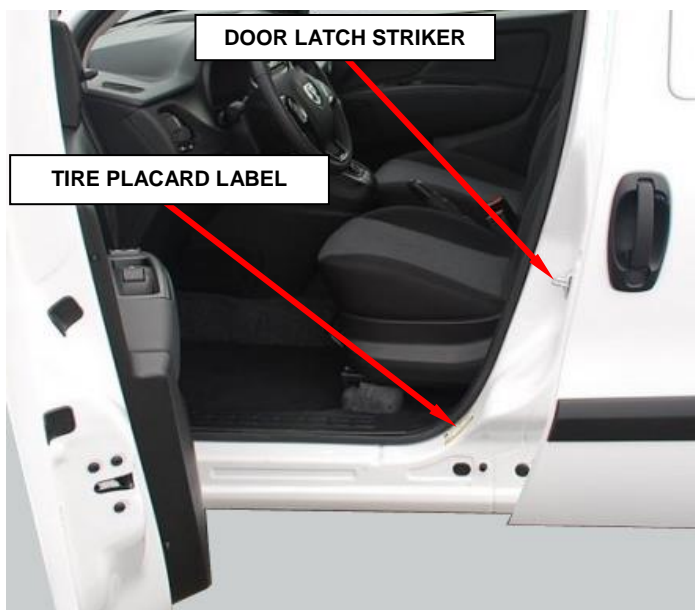
Figure 1 – Driver's Side "B" Pillar
