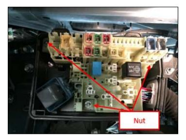
**7**. Release the fuse block locking clip that secures the fuse block to the fuse box.
