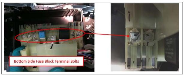
11. If any of the 8mm terminal bolts were found loose, the corresponding electrical connection needs to be visually inspected for damage. Was damage found to the electrical connection, harness or fuse block? If damage was found, contact TechAssist with documentation of the damage before replacing the harness.
