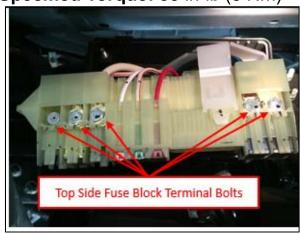
**9.** If any of the 10mm terminal bolts were found loose, the corresponding electrical connection needs to be visually inspected for damage. Was damage found to the electrical connection, harness or fuse block? If damage was found, contact TechAssist with documentation of the damage before replacing the harness.
