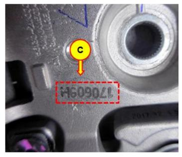
5. If the LOT No. (C) is not '170609H', reinstall all removed parts in reverse order of removal and finish the service procedure.
