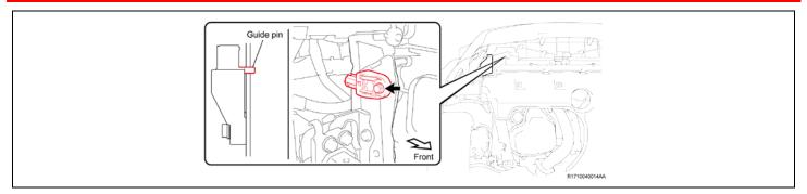
c. Engage the connector of the **NEW** front air bag sensor RH holding the sides of its yellow CPA (A click sound can be heard).
