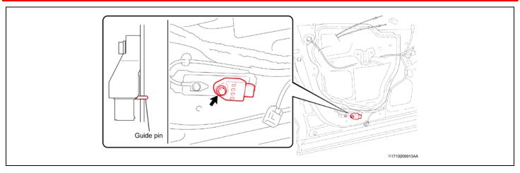
c. Engage the connector of the **NEW** front door air bag sensor holding the sides of its yellow CPA (A click sound can be heard).
