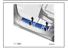
c. Disengage the 4 claws by pulling the rear door scuff plate straight up.
