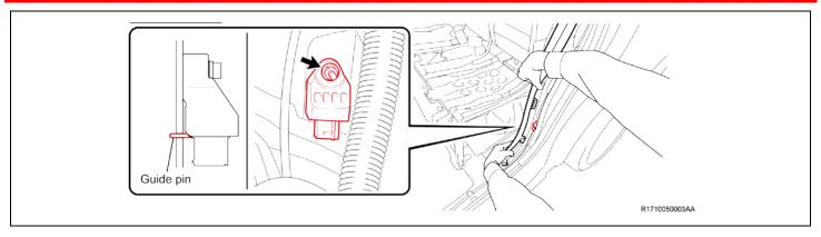
d. Engage the connector of the **NEW** quarter panel air bag sensor holding the sides of its yellow CPA (a click sound can be heard).
