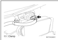
c. Disengage the clamp and disconnect the connector for the power seat.
