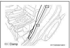
e. Engage the 2 clamps to reinstall the side trim panel.
