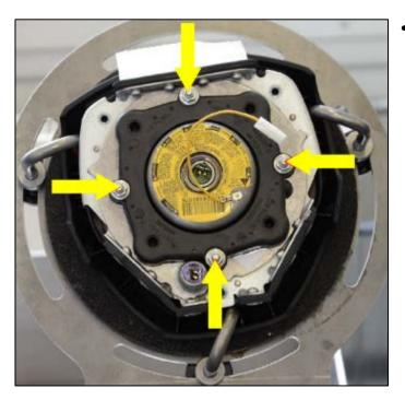
Install the new inflator and torque nuts <arrows> to 4.5 Nm
