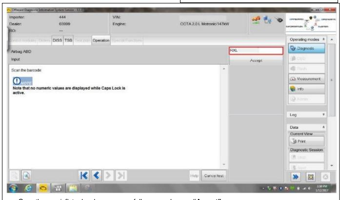
Once the new inflator has been successfully scanned, press "Accept"
