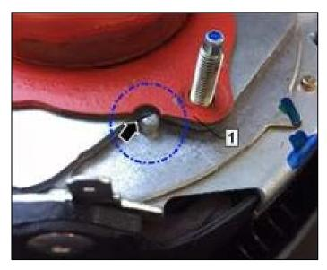
Install the new inflator onto the studs.
