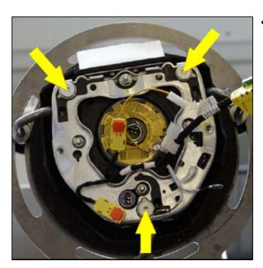
Install the horn ring and tighten the bolts <arrows> to 6 Nm.
