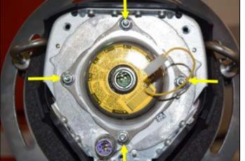
Install the new inflator nuts <arrows> and torque to 4.5 Nm.
