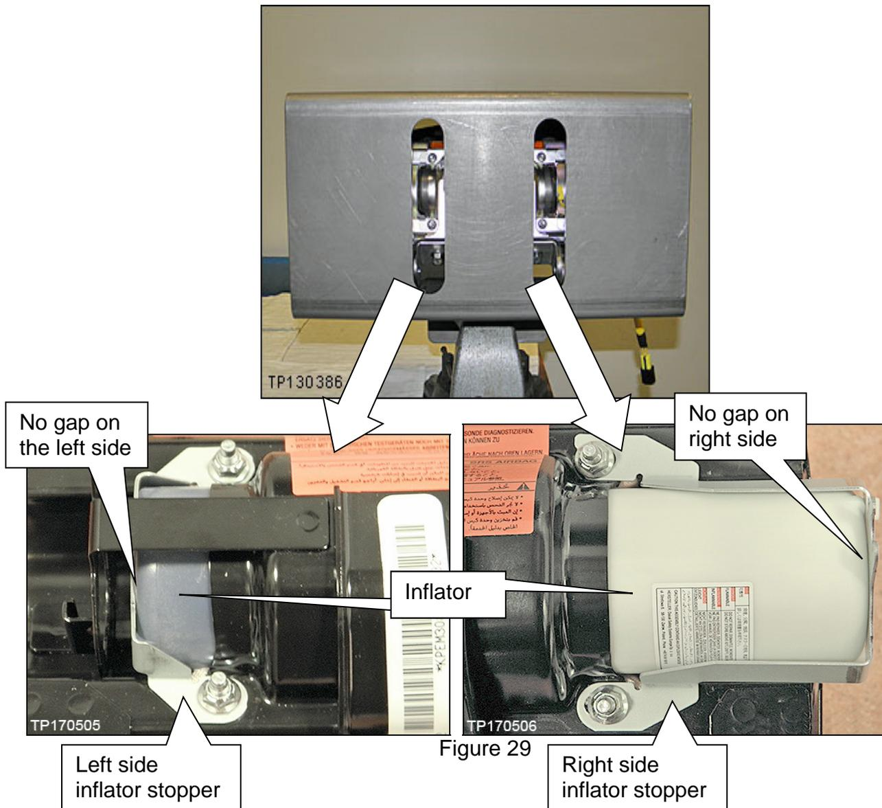
37. Torque the 4 inflator securing nuts.
