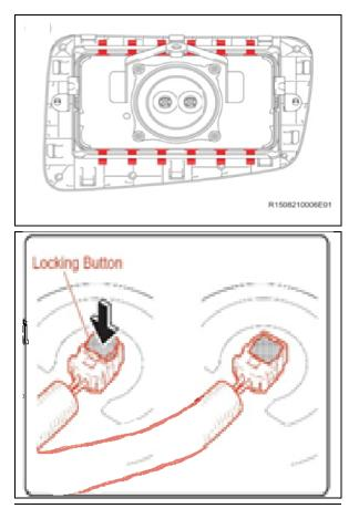
b) Reengage the tangs of the module into the door using the screwdriver with the shaft wrapped in tape.
