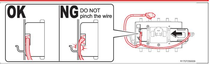
d) Insert the inflator with the correct orientation as shown in the illustration.
