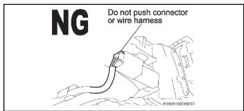
NOTE: When removing the register DO NOT push on the connector or wiring as it could be damaged.
