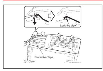
Removing the No. 3 air register
